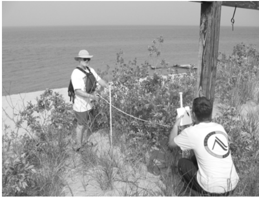
Figure 4 - Emery technique used to measure beach profiles.
