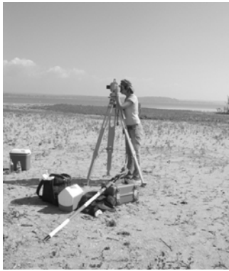
Figure 14 - EDM used to survey Sandy Pond Inlet
