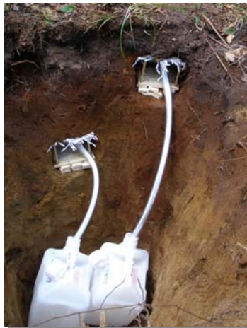
Figure 3: Wick lysimeters sampling soil moisture from two different horizons in an Adirondack soil pit.
