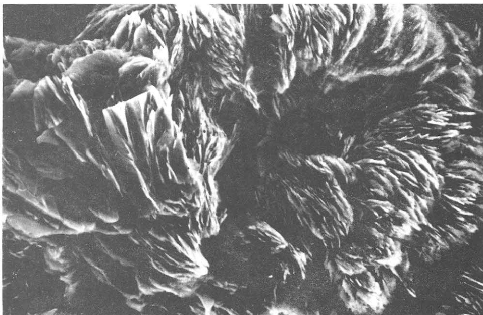
Figure 21. Creamy white aggregates of iron-rich talc crystals. The magnification of the SEM photomicrograph is about 700x. Photo by G. Robinson.
