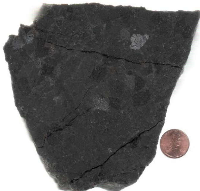
Figure 10. Cut slab of the Elmdale hornblendite displaying large, equant hornblende crystals.
