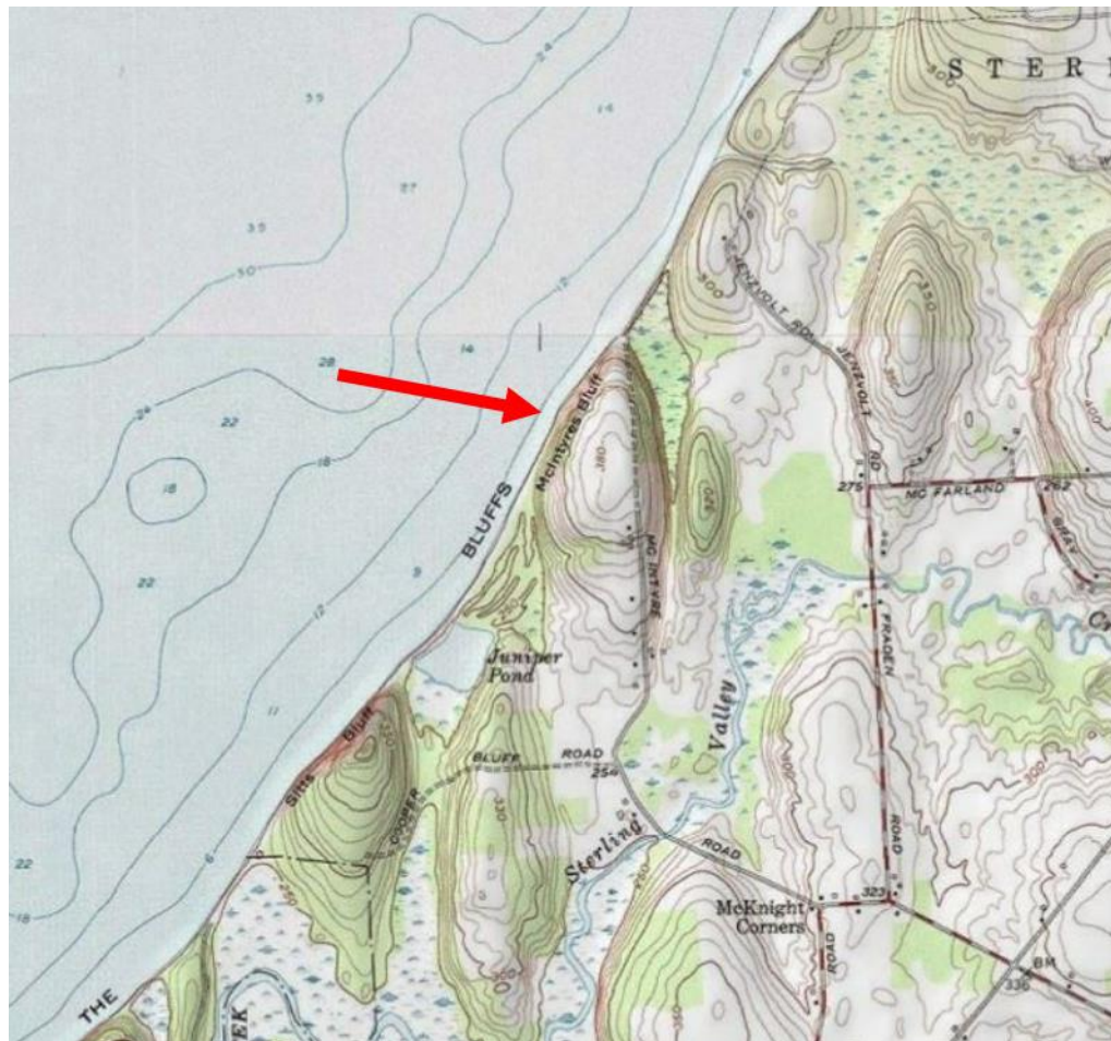
Figure 2. McIntyre's Bluff (red arrow) directly intersects the Lake Ontario shoreline. Erosion has exposed the interior of the drumlin, creating tall bluffs along the shoreline. These bluffs are composed of unconsolidated glacial till, which experiences intense erosion on a daily basis. Sitts bluff (west of McIntyre's Bluff) and Chimney Bluffs (off-map) have undergone similar erosional processes.
